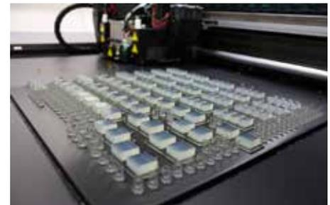
The perfusion tray was 3D printed in bio-compatible material since it will come into direct contact with cells and tissues.
