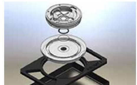
A 3D rendering of perfusion chamber's different parts
