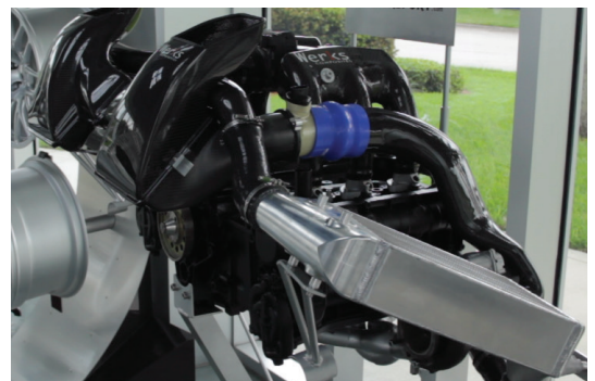
FDM soluble core-enabled components on a turbocharged engine.
