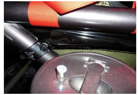
Triple Eight 3D printed the prototype of this seat mount in the racing car.
