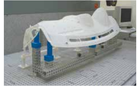
The CMM scan showed the ABS Prototype was within tolerance.
